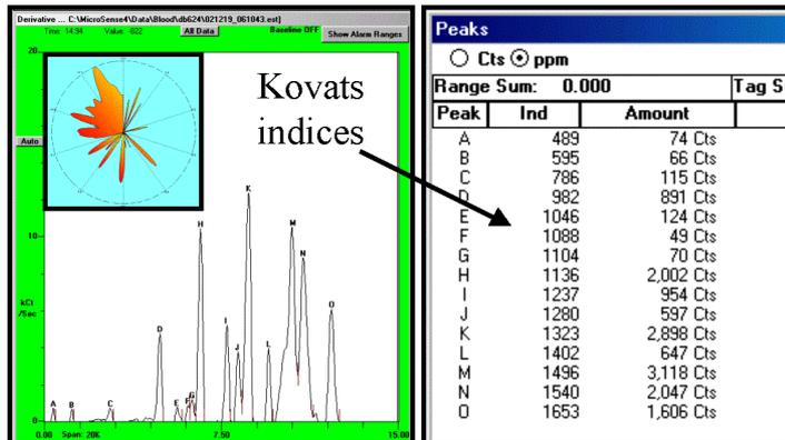
Figure 5- The derivative of odor intensity is a chromatogram used to determine chemical retention times. An analysis of odor from amino acid standards showing Kovats indices and odor concentration in counts.
