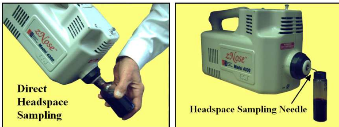
Figure 4- Sampling wine headspace vapors with the zNose.
