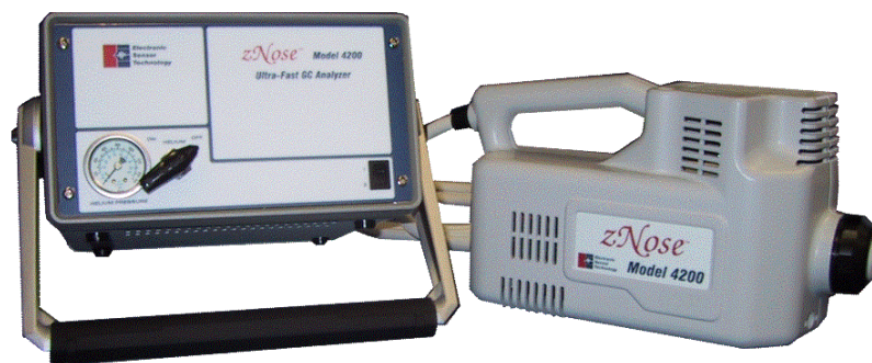
Figure 2- The zNose® is an ultra-fast battery powered gas chromatograph designed to quantify the chemistry of volatile organics over the range C4 to C24.
