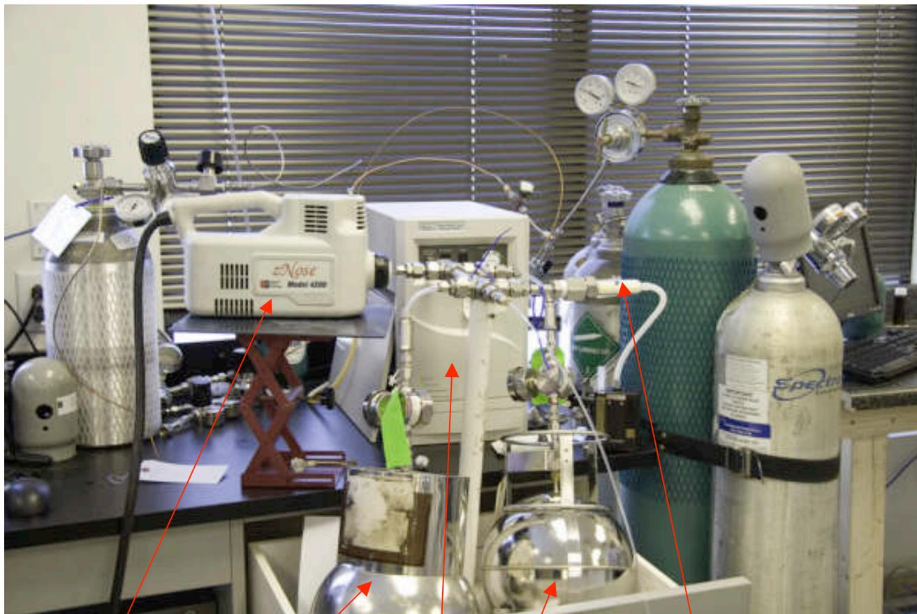
ZNose® Analyzer    TO-15 SUMMA Canister    TO-15 FSL Canister    TO-13 Cartridge
