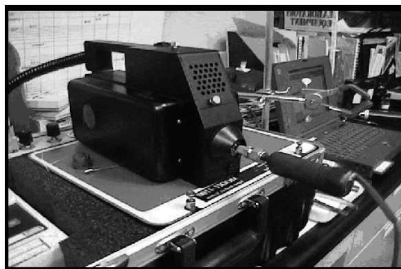
Figure 3- Desorbtion tool attached to fast GC/SAW
