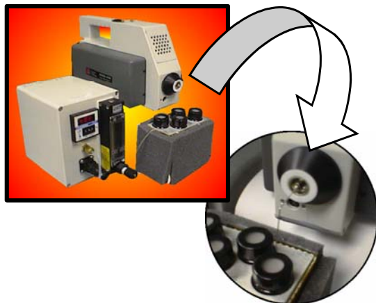
Figure 4- Handheld version of the zNose together with temperature controlled sample holder for 40 mL vials with sealed septa lids.
