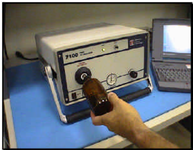
Figure 5- GC/SAW benchtop system contains an internal supply of helium carrier gas with capacity for more than 300 chromatograms. Sample pump, preconcentrator, and temperature programmed GC column are all controlled by an internal gate array processor which responds to the user's laptop computer connected by an RS-232 link.
