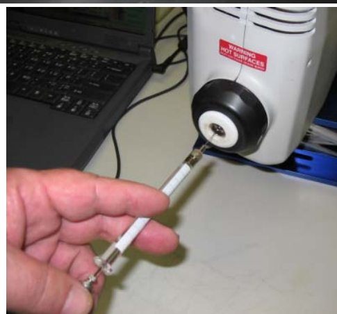
Figure 7- Calibration by directly injecting a known mass of phenol
