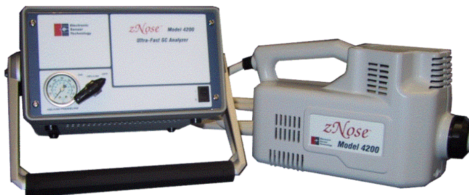
Figure 1- Portable zNose® technology incorporated into a handheld instrument.
