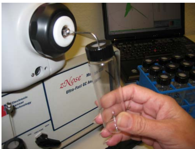
Figure 8- Testing samples in septa-sealed 40-milliliter vials.
