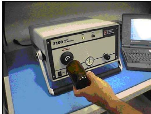
Figure 4- The model 7100 zNose® is a portable benchtop GC with an internal tank for carrier gas. Approximately 300 measurements can be performed with a single tank of gas. Both disposable and re-chargeable tanks are available.
