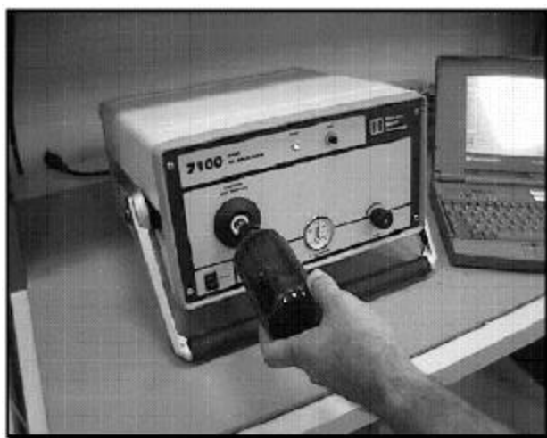
Figure 7- GC/SAW benchtop system contains an internal supply of helium carrier gas with capacity for more than 300 chromatograms. Sample pump, preconcentrator, and temperature programmed GC column are all controlled by an internal gate array processor which responds to the user's laptop computer connected by an RS-232 link.
