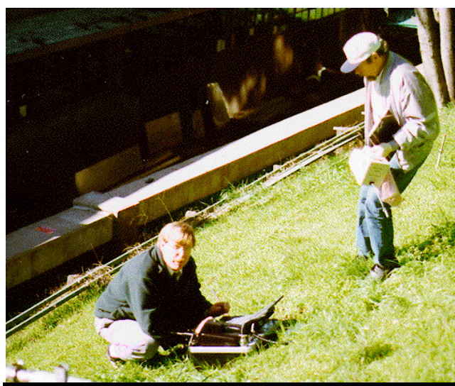
Figure 3 At the steeply sloping well-head gathering soil gas chromatographic data on migrating DNAPL contaminants.
