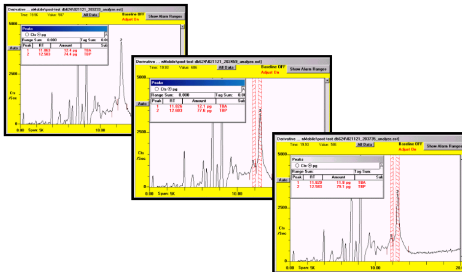
Figure 11- Replicate testing of wood headspace vapors demonstrating accuracy and precision of measurement.
