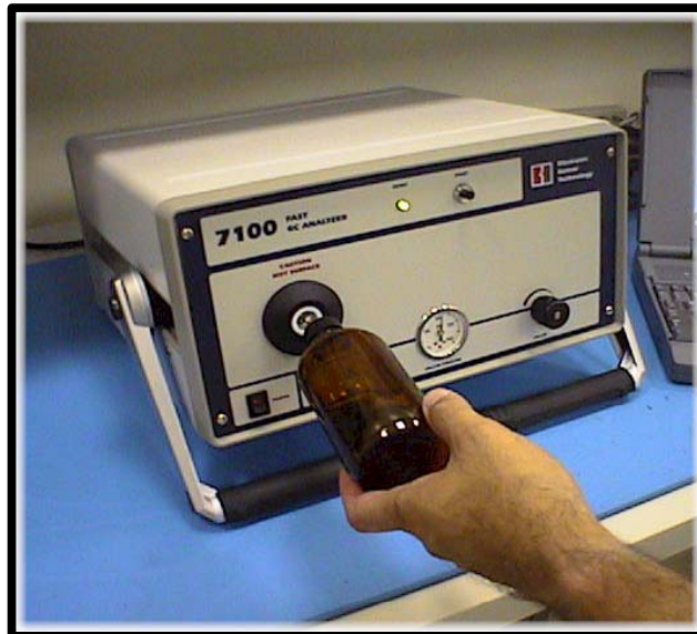
Figure 2- The model 7100 zNose uses a single benchtop enclosure which can also be integrated for unattended process control and monitoring.
