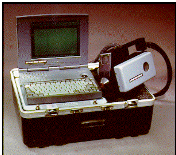
Figure 7- SAW/GC Field Screening Instrument.
