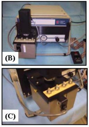
**Figure 4.** The zNose® ultra-fast GC design (A) reconfigured as fully automatic chemical process controller (B & C) with a selectable multi-port inlet for measuring and controlling up to 16 multiple vapor sources.
