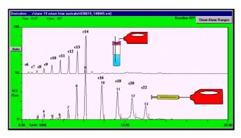
**Figure 5.** Typical n-alkane chromatogram response of a GC/SAW system
