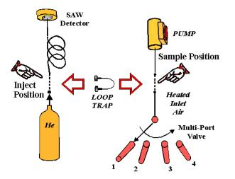
**Figure 1.** Multi-port process control system containing one section with helium flowing through a self-heated capillary column and the other for sampling up to 16 different vapor sources.
