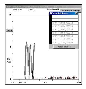
**Figure 7.** Replicate MIC chromatogram measurements, horizontally offset, using 55 ppbv vapor standard. Sample time was 30 seconds (15 milliliter) and detector temperature 20°C.
